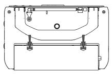
2.) Remove the coiled AC cord form the storage compartment and extend it to its full length.
